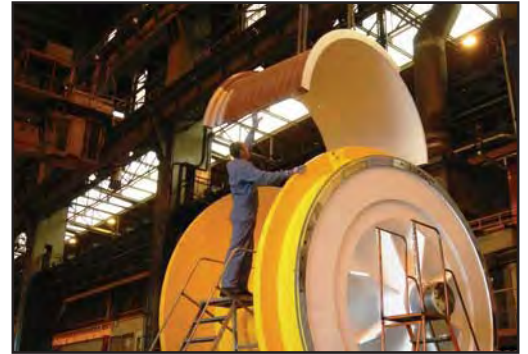
Lebus can produce split sleeves for the very biggest winch drums
