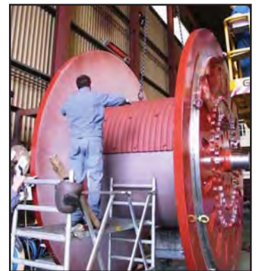
Split sleeves are an effective and economical solution for providing Lebus grooving onto worn old drums. They can be retrofitted either on site or in the customer's own workshop
