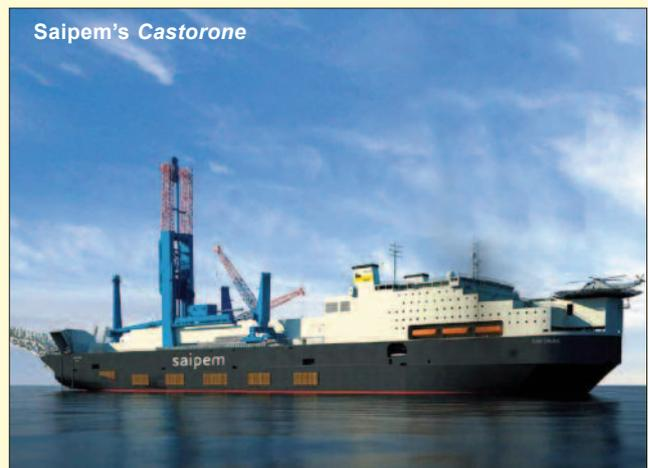
As the winches are turned, the vessel moves towards the anchors, laying down pipeline at the back as it moves forward. A dynamic positioning system keeps the 330m-long vessel steady at all times.
