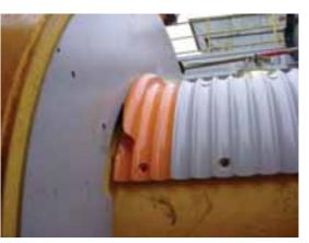
Welding or bolting a grooved sleeve onto a smooth drum can be a cost-effective alternative to total drum replacement
