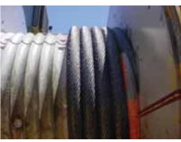
Parallel grooving on a winch drum...
