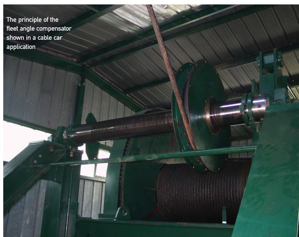
spooling devices are available. One is a fleet angle compensator, which is driven automatically by the rope tension. The other is a level winder that is mechanically driven. Both offer a solution to guide the cable along the drum between flanges, but each has its advantages and disadvantages.
