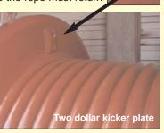
crossover sections, the rope is given a kick after each complete wrap to take its proper position on the pattern.
