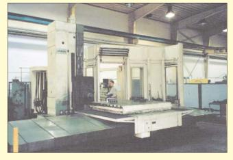
The new five-axis CNC horizontal boring table
