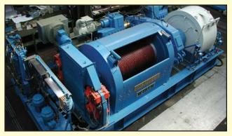
A Wirth GH 3000 draw-works, similar to – but half the power of – the new GH 6000 that is now being developed
