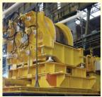
International Engineers GmbH delivered a pair of grooved split drum sleeves. The drum is 2690mm diameter and holds up to five layers of Redaelli 120mm diameter galvanised steel rope, one of the biggest non-rotating wire ropes ever made.
