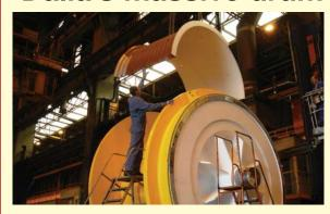
This is the drum of the 405-tonne winch on Total Fina Elf's new Dalia FPSO vessel.
