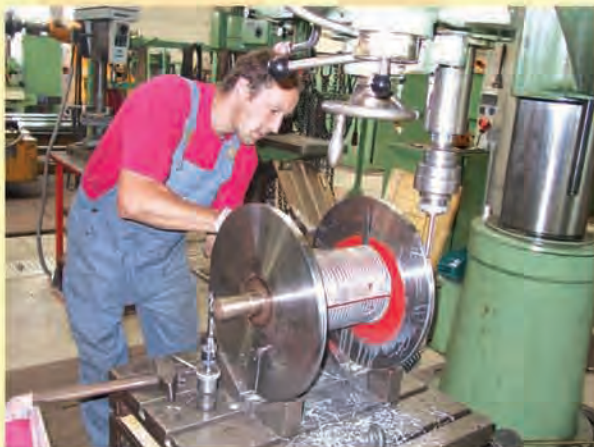
Lebus公司在德国的工厂里生产绳槽卷筒和绳槽衬套。 Lebus manufacturers grooved winch drums and drum sleeves at its factory in Germany.
