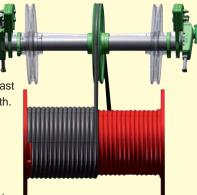
If spooling in multi layers, the drum must have Lebus grooving. For a single layer, helical grooving will also work.
