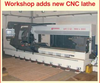
Despite the current difficult economic climate, Lebus continues to reinvest in the business. It has recently installed in its main workshop a new Iberimex-Geminis CNC turning lathe with a special control unit for forming both parallel and helical grooving. It has the capacity to work on tubes up to 1000mm in diameter, 3000mm long and up to 4800kg in weight.
