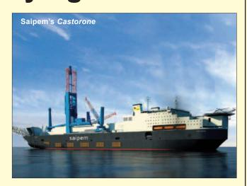
As the winches are turned, the vessel moves towards the anchors, laying down pipeline at the back as it moves forward. A dynamic positioning system keeps the 330m-long vessel steady at all times.
