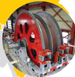
Hong Kong Peak Tram • Wire rope drum • 5,058 mm 1 • 843.5 mm 2 • 50.5 mm 3 • 1,365 m 4 • 1,200 m track • Speed 6 m/s • 120 passengers/trip
