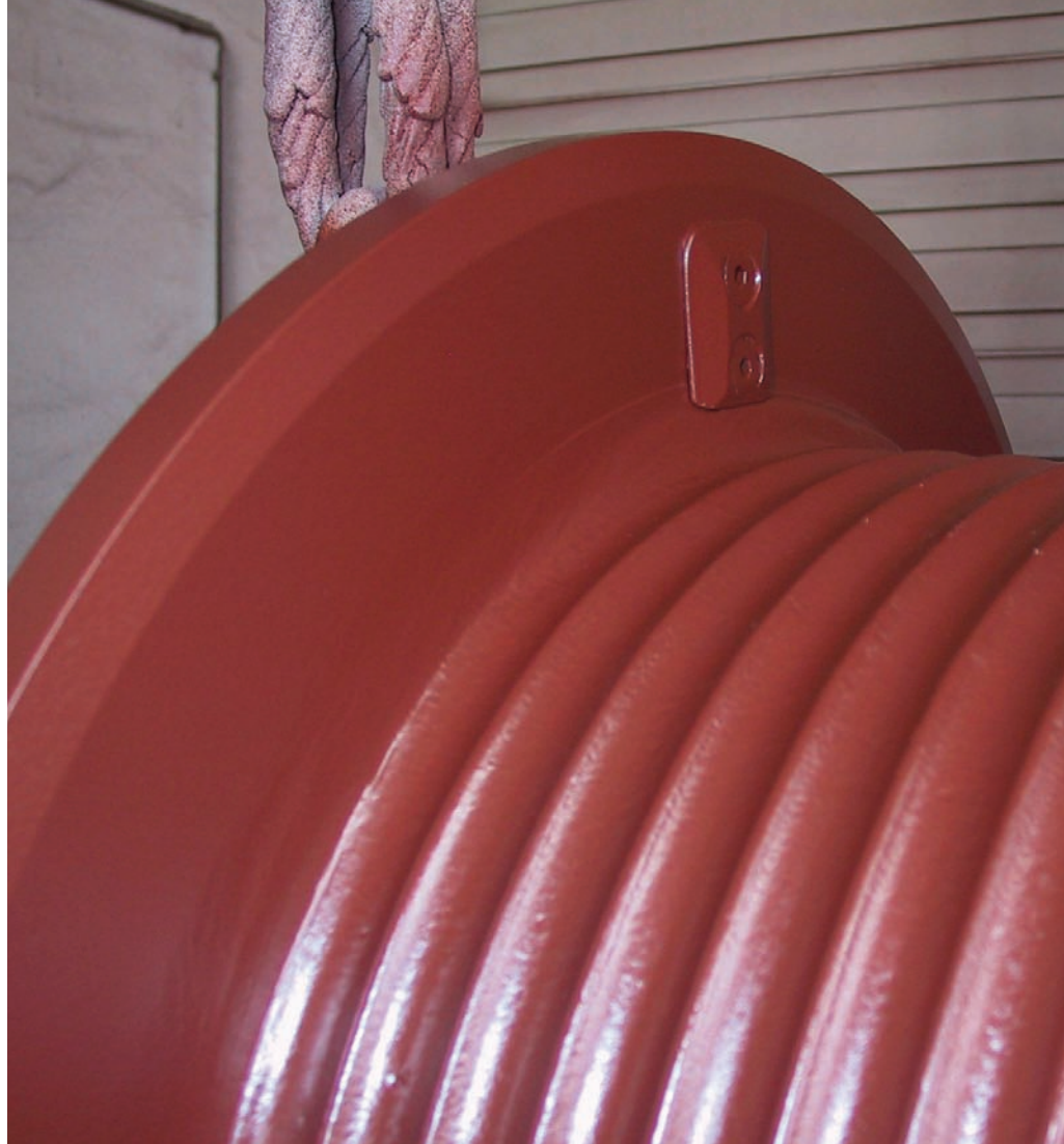
A "two dollar" solution is a kicker plate on the flange of the winch drum
